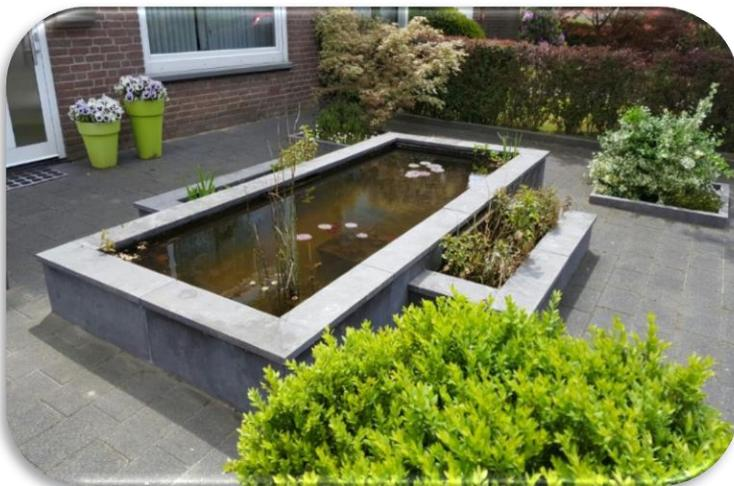
**VB-EPDM** prefab planters are available in almost any shape and size. They are easy to install in existing planters, but they can also be used as self-contained planters in green areas. VB-EPDM sheeting is resistant to root penetration in accordance with FLL guidelines. However, it cannot hold back some roots, for example the roots of certain bamboo and reed-like plants, for which alternative arrangements must be made. VB-EPDM sheeting is UV-resistant and does not leach out.
